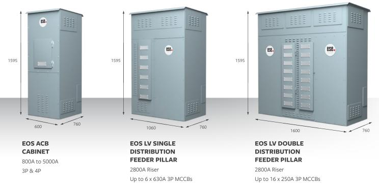
\* All dimensions measured in mm. The EOS Range is tested at 50kA / 1 sec IP33.
